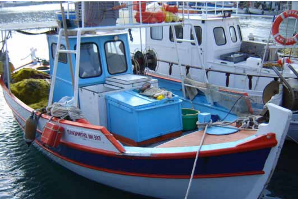
Figure 7 (Left side): Trehandiris used as small scale fishery boats. Photo: Argyris Kapantagakis.
